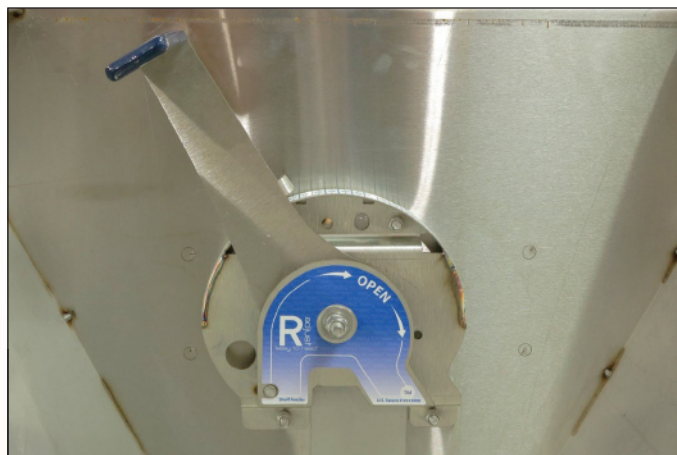
The R adjust is easy to operate for extreme accuracy and infinite control of feeder settings.
