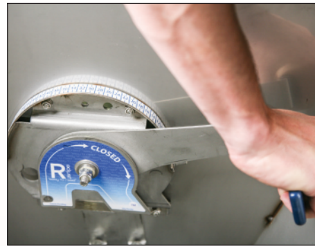
The R adjust system is easy to operate for extreme accuracy and infinite control of feeder settings.
