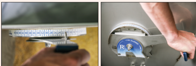
The R adjust system's innovative numeric dial indicates the precise setting for opening and closing the feeder.
