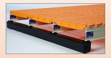
Fiberbeams come in a range of sizes. To best meet the specific needs of your buildings, Farmweld offers a range of different beam sizes, with standard sizes of ½" x 3" (6 mm x 76 mm) and ½" x 5" (6 mm x 127 mm). For added durability, fiberglass beam clips protect the fiberglass beam from wear and tear.
