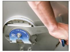
The R adjust system is easy to operate for extreme accuracy and infinite control of feeder settings.
