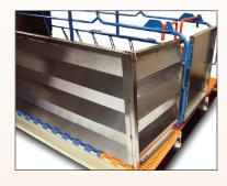
Creep-area dividers are made of corrugated stainless steel. Piglet creep-area dividers are 20" (508 mm) tall. Framed dividers on the row ends are 24" (610 mm) tall to prevent sows from jumping.
